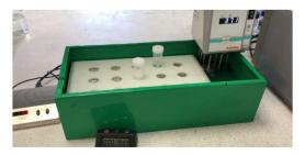
**Figure 2. Incubation Method 1.** Samples ( $\sim$  0.5 g) in 40 mL, 30 x 84 mm polypropylene tubes in a designed polypropylene tube holder (Megazyme cat. no. **D-PPSTH**) [C(w)] on a 2mag Mixdrive 15<sup>®</sup> submersible magnetic stirrer in a custom made water bath (Megazyme cat. no. **D-TDFBTH**). This arrangement allows stirring of 15 samples at controlled speed (170 rpm) and 37°C.
