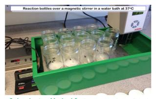
**Figure 3. Incubation Method 2.** Samples ( $\sim$  1.0 g) in Fisherbrand bottles on a 2mag Mixdrive 15<sup>®</sup> submersible magnetic stirrer in a custom made water bath (Megazyme cat. no. **D-TDFBTH**). This arrangement allows stirring of 15 samples at controlled speed (170 rpm) and 37°C.
